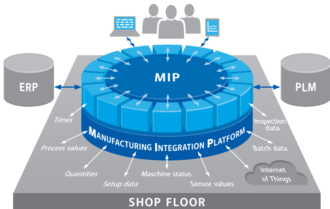
Figure 1: The Manufacturing Integration Platform (MIP) as an open link between shop floor and production-related IT applications
